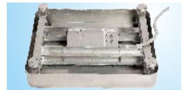
Platter with frame work assembly
