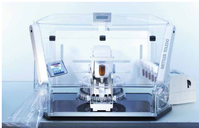
1-to-30 dosing system in safety enclosure QSE1
