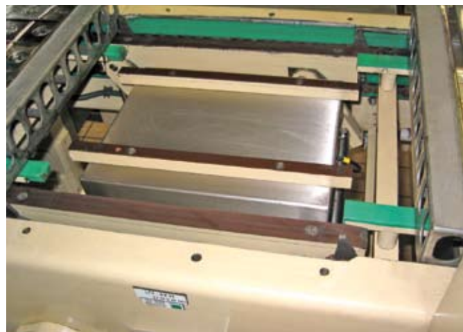
5kg chocolate bars: net content control with METTLER TOLEDO platform integrated into the conveyor (see picture below)
