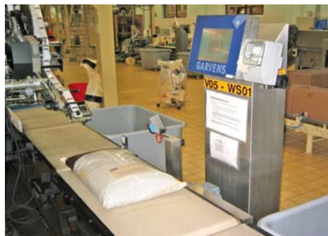
25kg chocolate pellets bags: 100% net content control by dynamic METTLER TOLEDO Garvens checkweigher
