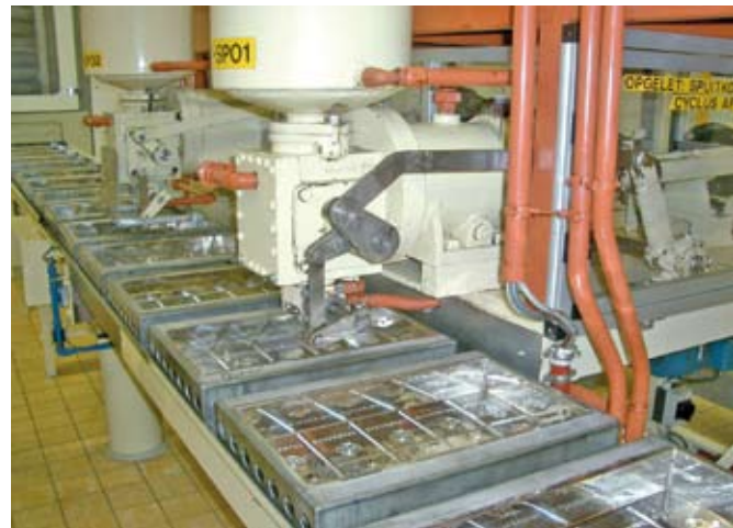
5kg chocolate bars: net content control with METTLER TOLEDO platform integrated into the conveyor (see picture below)
