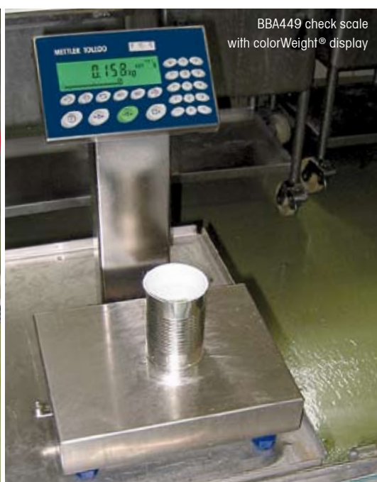
Automatic rejection of underweight cans
