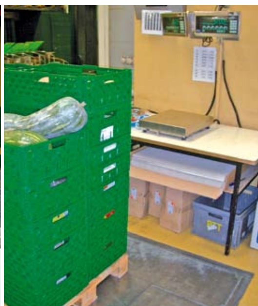
Precise and time-saving net weight determination with IND690Sys weighing terminal and PBA430 platform
